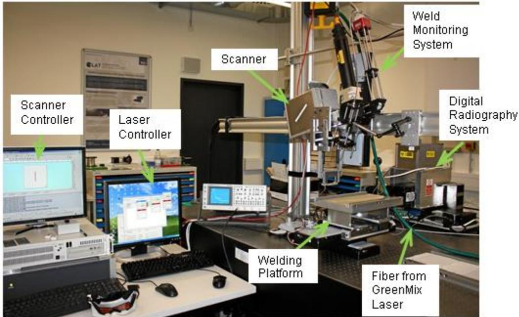
**Figure 4** Dual wavelength test platform for solar module application (Courtesy of RUB).
